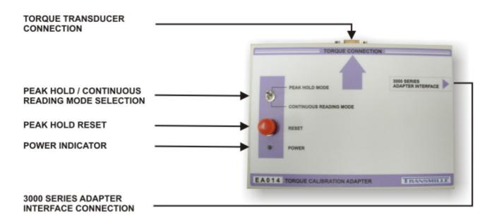
Once connected, the power LED on the EA014 adapter will illuminate. This adapter is now ready for use using the ProCal calibration software (operation detailed separately)
